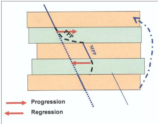
Figure 3. Pressure regression due to communication between the deeper compartment and shallow ones.
