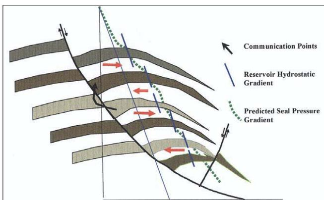
**Figure 7.** An example of geopressure profile development due to communication across growth fault.
