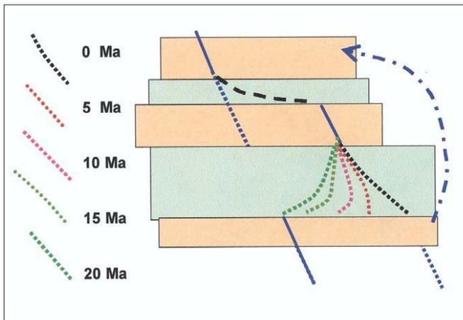
Figure 5. Pressure decay in a regressive geopressure system, over the course of time. The communication passage is the blue dashed line. Notice that MPP and the PPP differences are a function of time. Permeability in the seal dictates the rate of decay.
