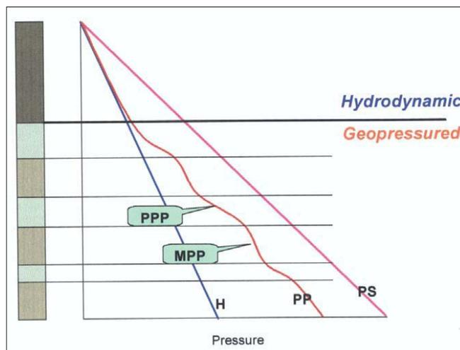
Figure 1. The two main subsurface pressure subdivisions—the normal pressured hydrodynamically active upper section and the compartmentalized geopressured lower section. Hydrostatic, pore pressure, and principal stress are represented as H, PP, and PS, respectively. Pore pressure in the seal and reservoir are PPP and MPP, respectively.
