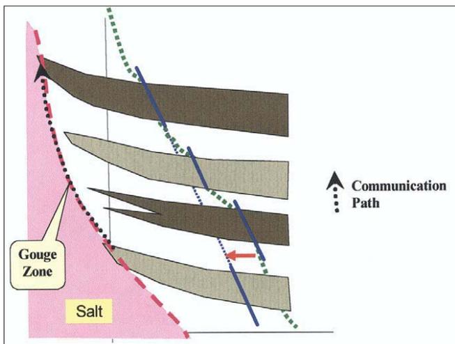
**Figure 8.** Cross-section on a flank of salt basin. Communication takes place along the salt-sediment gouge zone. Notice pressure progression in progress with depth where beds are pinched out before reaching the gouge zone. On the other hand, regression and large PPP/MPP difference takes place where structural failure exists and communication occurs.
