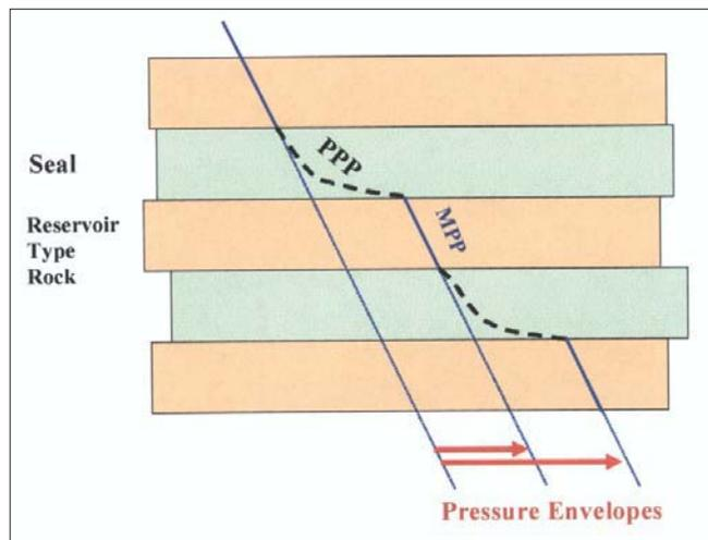
Figure 2. MPP cascade fashion progresses with depth in active sedimentary basins.
