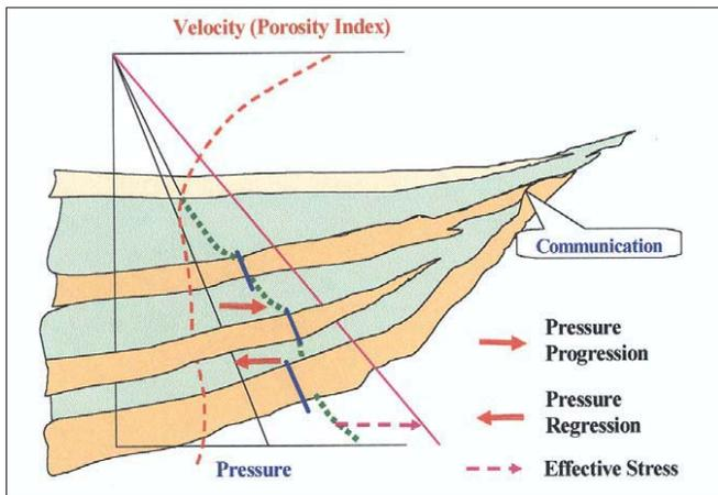
**Figure 6.** Cross-section showing the effect of the geometry of deposits and facies changes on the subsurface geopressed profile. Note non-alignment between MPP and PPP at the lower compartment.
