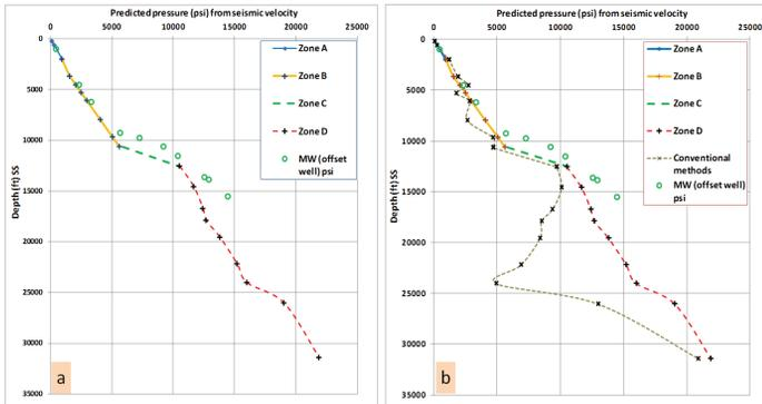
**Figure 8.** The before drilling predictive pressure model for the four zones is shown on the left plot (a). A comparison between the conventional and the newly proposed method is displayed on the right plot (b). Open green circle represents the mud weight that was used to drill a nearby offset well and also calibrates the pre-drill model. Note the ~5000 psi pressure ramp at zone C.
