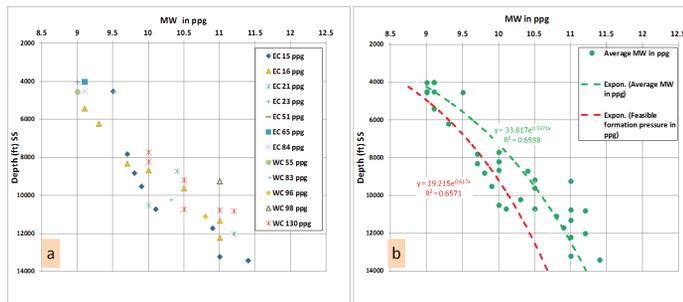
**Figure 6.** Mud weight used to drill twelve wells in zone B of East and West Cameron areas. It shows an average pressure gradient increase with depth from 9.5 to 11.5 ppg that combats a hydrodynamic flow, and is not a normal hydrostatic pressure (8.9 ppg). Plot (a) represents mud weight (ppg) records in zone B (Middle – Upper Lower Miocene) of all wells in an inner shelf depositional environment. Plot (b) shows the calculation method of average ppg for MW and FFP.
