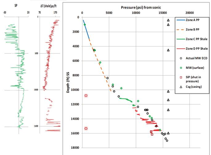
**Figure 9.** Calibration criterion during drilling MWD – pore pressure (PP) of the before drilling seismic-pressure model is shown. Zones A PP (blue) and B PP (orange) are calculated (equations 2 and 9). Zones C PP shale (green) and D PP shale (red), MW, SIP, and Csg are predicted shale pore pressure from sonic (LAS), mud weight (surface and equivalent circulating density), shut in pressure and casing seats respectively.
